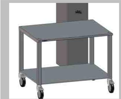
Position the wheeled stand in the installation location and level it so that the absolute tilt of the appliance in operation does not exceed 2° (3.4%).
