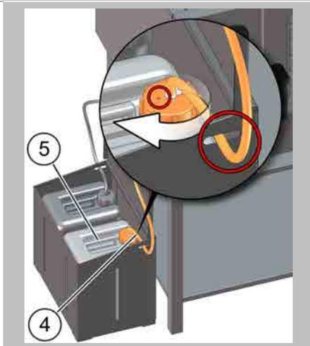
Insert the suction nozzle on the red extractor tube into the cleaning-agent canister (5). There must be no kinks in the tube and the vent hole in the canister must be open and unblocked.
