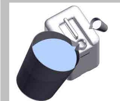
Mix the supplied ConvoCare Kconcentrate with soft water in the empty ConvoCare rinse-aid canister. Follow the instructions in the user manual on mixing the ConvoCare rinse aid in the canister.
