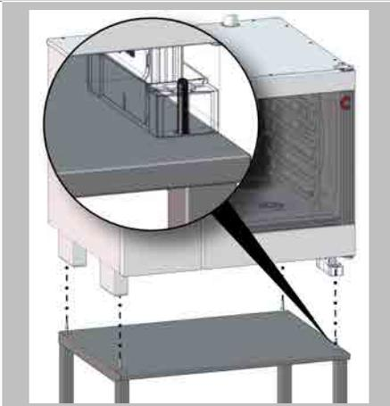
Position the appliance on the stand. Make sure that all four bolts are guided into the locating holes in the appliance feet provided for the purpose.
