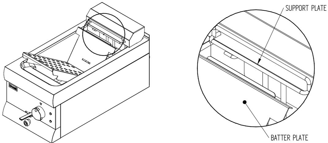
**Do not attempt to lift the element without first removing the batter plate.**
