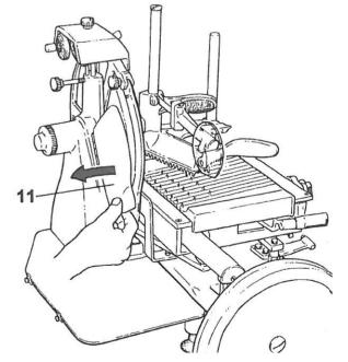
Remove the blade protection 10 after loosening the locking knob.
