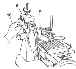
Lower the sharpener 8 back carefully, the blade will be automatically centered between the two grinding wheels.
