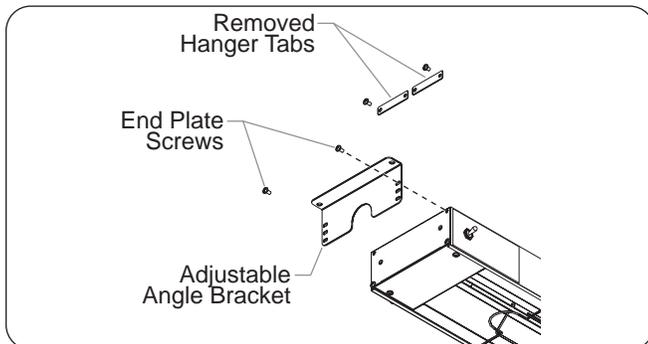
Figure 21. Aluminum Model Adjustable Angle Bracket Installation
