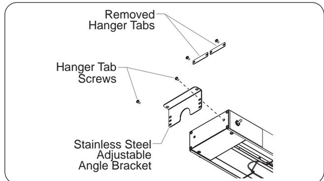
Figure 23. Stainless Steel Model Adjustable Angle Bracket Installation
