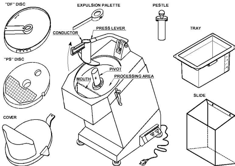
Fig. n°28 - View of the machine dismantled for cleaning
