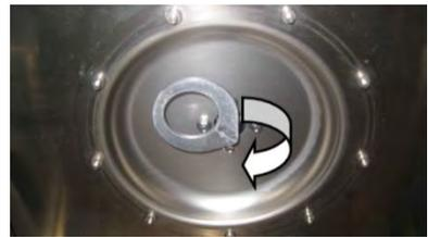
*Remove the remains of the old gasket before fitting the new impincher plate (comes with gasket).*
