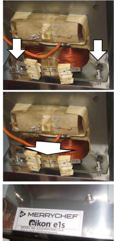
**Fitting a transformer (high voltage)**
