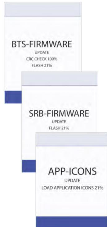
9. On completion, the start up screen is displayed showing the updated firmware versions before moving to the pre-heat temperature screen.
