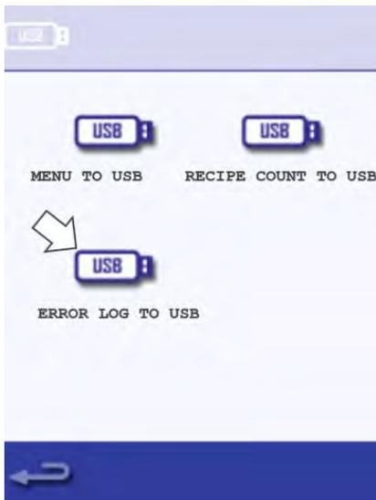
5. Select the green check mark to copy the error log to the USB memory stick. The upload progress is shown followed by the upload status.
