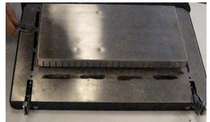
4. Apply sealant around the existing door seal area. Ensure you do all four sides.
