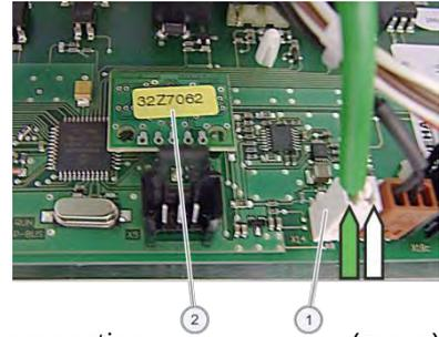
Ensure the thermocouple negative (-) connection (white) and positive (+) connection (green) are fitted the correct way round or the oven temperature readings will be wrong.
