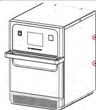
3. To remove the rear panel, first unscrew the three screws at the bottom of the panel and then the two screws either side of the air duct grille.
