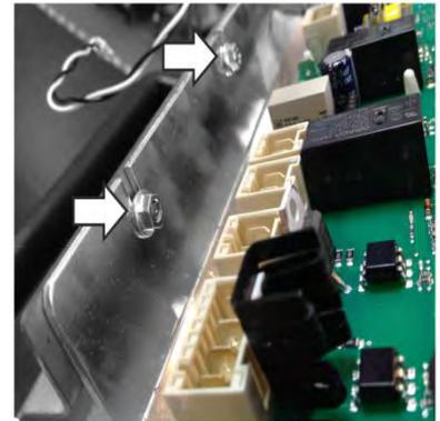
3. Remove the PM (Personality Module) from the SRB and place safely aside.
