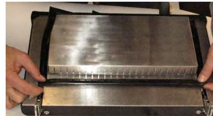
6. Apply sealant underneath the door seal and press down firmly to tightly secure the door seal onto the door. Ensure it is straight and wipe off any excess sealant leaking.
