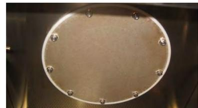
2. The partition plate features a rubber gasket on its upper side which adheres to the upper surface of the cavity.
