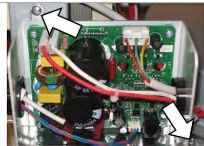
3. Slide the board/backing plate towards the rear of the appliance to provide access to the cooling fan.
