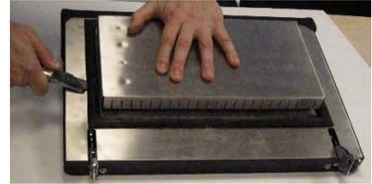
2. Gently pull the metal clip out of each corner and lift off the door seal
