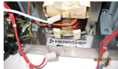
2. Disconnect the transformer(s) from the magnetron(s) by unplugging the orange cables at the magnetron(s).
