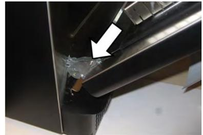
3. Close the door onto the two metal pins and then free the door by pulling upward and forward. The door should now be fully removed.
