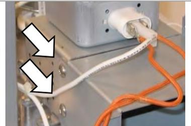
2. Disconnect the orange and white cables from the magnetron body.
