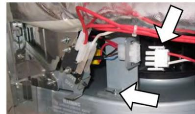
2. On the left-hand side of the appliance, unfasten the PZ2 and M7 nut that hold the convection fan motor speed controller board backing plate.
