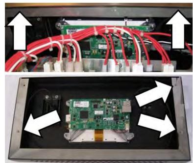
4. Unfasten the four M5.5 hex head flange bolts to remove the QTS assembly from the front panel.
