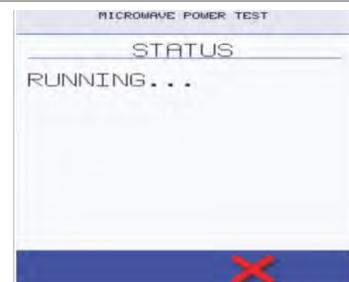
6. When the countdown has finished, remove the container from the cavity. Immediately stir with a plastic implement and measure the water temperature.
