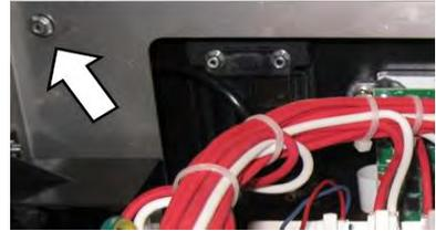
3. Remove the top front panel (including the touch screen and QTS assembly) from the frame of the casing by lifting upward and towards the front of the appliance. Note the three studs in corners of the assembly that locate and hold the assembly to the appliance body.
