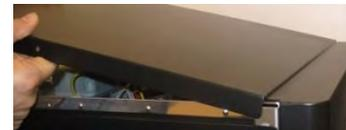
2. To remove the side panels, unscrew the two screws that attach each side panel to the rear panel.
