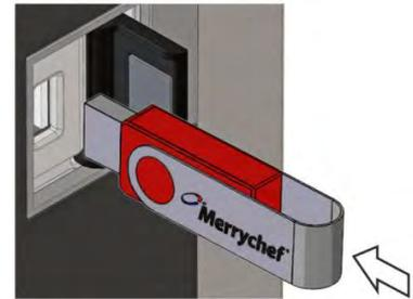
6. Once the USB memory stick has stopped flashing, select the 'Menu to Oven' symbol.
