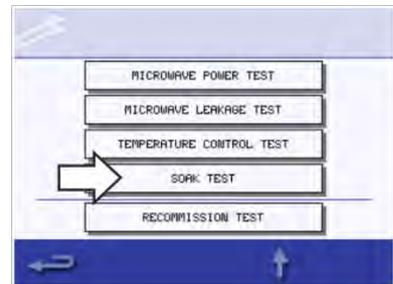
3. Run the test (30 minutes at maximum oven temperature, 50% microwave power, and maximum fan speed), carefully checking the appliance casing, joints and door seal for signs of steam or water escaping from the cavity.
