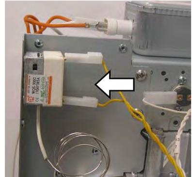
The thermostat uses a temperature sensor which is pinned within a holder located towards the rear of the top left edge of the cavity.
