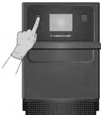
2. Preheat the cavity. Once reaching the preset operating temperature it will take about 30 minutes to cure the protective chemical.
