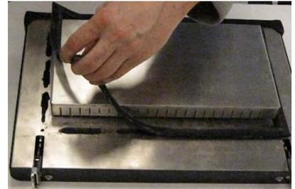
3. Remove excess sealant using the stanley knife or similar to make the surface as flat as possible and then clean the inner surface area wiping off any remaining sealant and residue.
