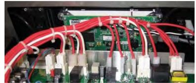
2. Unfasten two M7 hex head flange bolts to remove the SRB from the frame of the casing.
