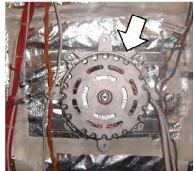
The element connections can be seen to the left of the convection motor.
