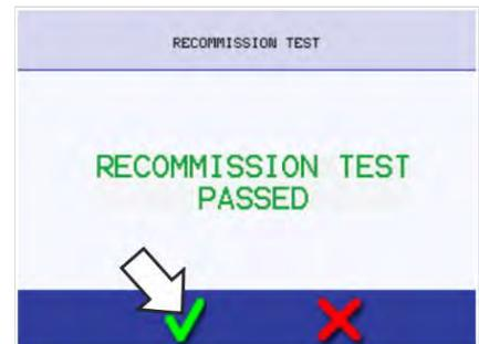
4. When all the tests have been successfully performed the display shows the Recommission Test has passed. Select the green check mark to confirm.
