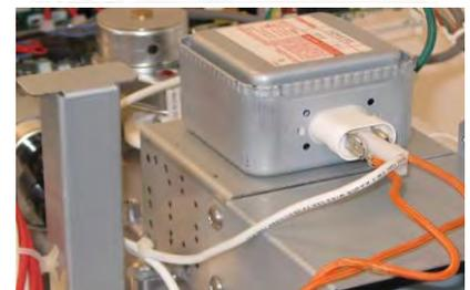
3. Using the DMM, test the insulation resistance between:
