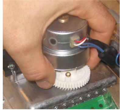
The stirrer can then be removed by turning clockwise.
