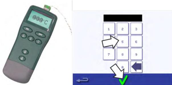
5. Retest to check that the cavity temperature reading is the same as the oven maximum set point temperature.
